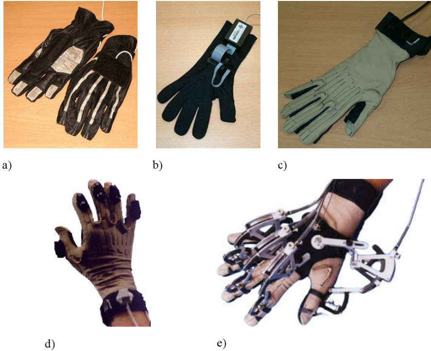
Fig. 1. Guantes de datos. a) FakeSpace Pinch Gloves b) Fifth Dimension Data Glove c) Immersion CyberGlove d) Immersion CyberTouch e) Immersion CyberGrasp
